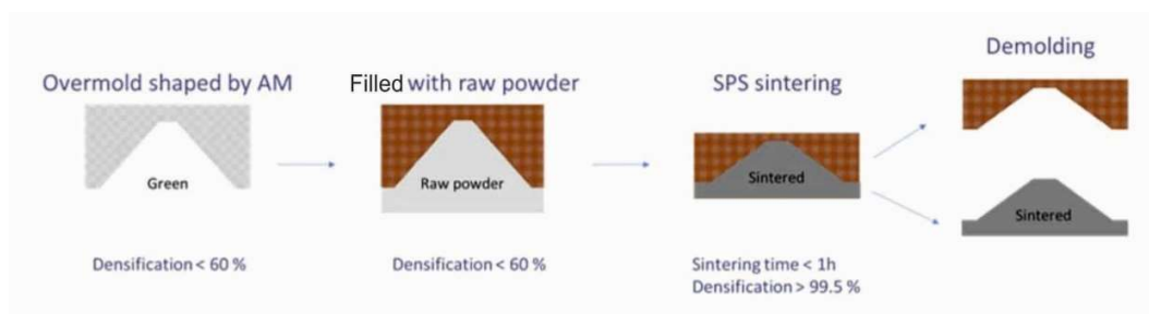
Figure 22: Schematic sketch of the counter-form method (Courtesy of Norimat SAS).
