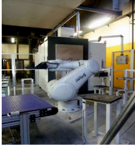
Figure 11: Example of automated stacking and manipulating of a Dr. Fritsch FAST/SPS sinter press by means of a 6-axis robot. (Courtesy of Flertex Sinter).
