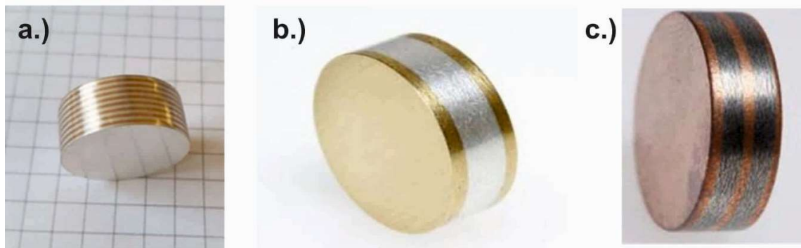
Figure 35: a.) Multilayer structure b.) Sandwich structure of silver-copper c.) Combination of copper and molybdenum in multilayer arrangement (Courtesy of RHP Technology GmbH).
