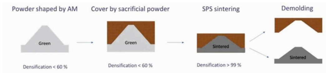
Figure 20: Schematic sketch of the preform method combining additive manufacturing and FAST/SPS for the production of complex shaped parts (Courtesy of Norimat SAS).
