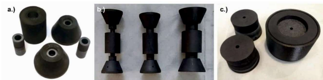
Figure 14: Examples of graphite tools a.) Die, punches with holes for pyrometer, cones for adaptation to the electrodes b.) Tools in laboratory scale with diameter of 12, 20 and 30 mm and c.) Tools for larger FAST/SPS with diameter of 100 mm.
