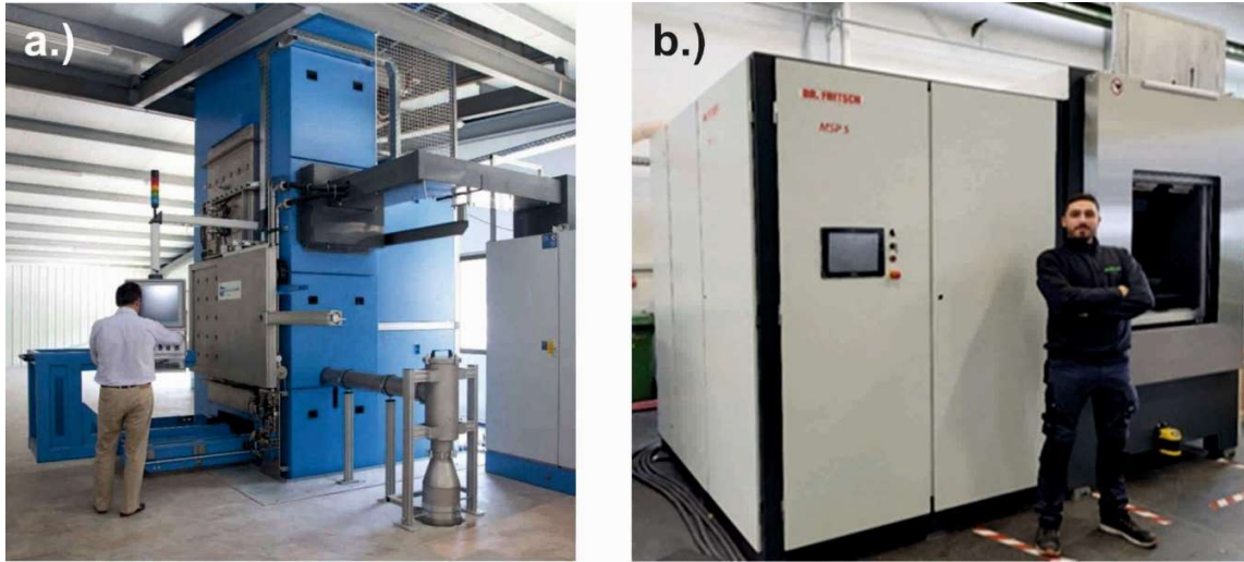
Figure 7: Examples of FAST/SPS devices for production of parts with diameters up to 450 mm a.) KCE®-FCT H-HP D 400 from FCT Systeme GmbH (Courtesy of FCT Systeme GmbH) b.) MSP5 & MSC5 from Dr. Fritsch GmbH (Courtesy of Dr. Fritsch GmbH).
