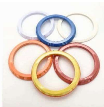
Figure 32: Watch bezel made of coloured ceramics (Courtesy of Norimat SAS).
