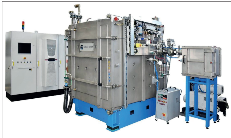
Fig. 6 Batch furnace, specially equipped for thermal processing of SiSiC 3D screen printed parts
